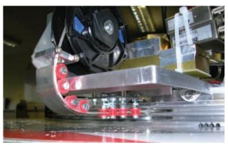
Fig. 5 Cable reel and guides on exterior side of azimuth rail.
