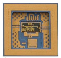
Fig. 5 The fabricated RFIC integrated into an existing multilayer LTCC module.
