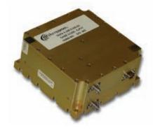
Model SSPA 0.225-2.000-50 is a high power, broadband GaN amplifier that operates from 225 to 2000 MHz minimum. It is designed for harsh environments such as munitions and high performance fighter aircraft. Power added efficiency in saturation is typically 40 percent across the band. Input VSWR is 2.0:1 maximum. Output VSWR is 2.0:1 typical. This unit is equipped with Aethercomm's proprietary DC switching circuitry that enables and disables the DC-DC circuitry in
