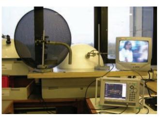
▲ Fig. 8 Receiving satellite TV at 11 GHz.
