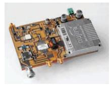
Fig. 6 Nujira HAT power modulator integrated with a typical PA.
