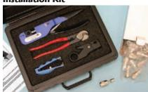
The RFA-4511 series is a comprehensive installation kit series for crimping N-type connectors onto LMR-400® or equivalent cables. The kit combines a cable cutter, one-step cable stripper, the Cable Devil® preparation tool, professional grade crimp tool and die, and 25 N male connectors. All are housed in a rugged, foam lined case with installation instructions.
