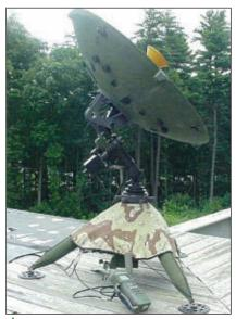
A Fig. 4 Transportable Ka-/Ku-band Sat-Com antenna system.
