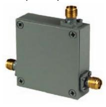
This small footprint diplexer is designed for the DC to 2000 MHz band. This diplexer features lowpass rejections of 60 dB minimum from 1200 to 2000 MHz and highpass rejections of 60 dB minimum from DC to 800 MHz. This compact mechanical package is rated at 10 W input power, features SMA connectors on all ports, high broadband isolation and wide frequency ranges. High power models are also available. Standard delivery: five to six weeks.
